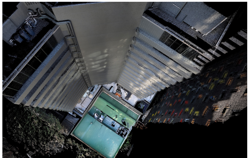
This building scan is colorized with realistic colors and texturized to produce an intuitive element in a city model.
